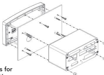
Drill standard holes for easy, quick installation
