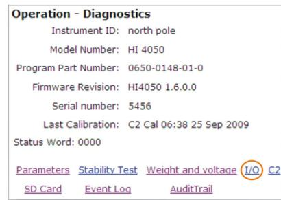
I/O reads 1. If an Input or Output is not in use, the I/O reads 0. In our example none of the inputs (User Switches) are being used so they all read 0.
