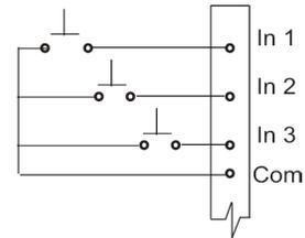
These standard inputs cannot interface with 24v logic directly. To activate the input contacts sent from a PLC, it is necessary to install a relay device as the dry contact or install the optional digital I/O card.
