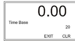
Step 2. To set the Time Base, use the left or right arrow to position the cursor and the up or down arrow to select the values. Our example uses 20.
