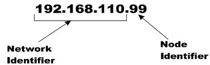
If your Windows PC already had an IP address assigned, simply increment by one the Node Identifier field of the IP Address you wrote down in the Windows PC configuration steps above. If your Windows PC was originally set to automatically obtain an IP address (DHCP), use 192.168.100.50 for the HI-4050 IP address in step 3 below.
