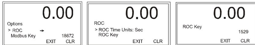
Step 2. Use the left or right arrow to position the cursor and the up or down arrows to select the values; then press Enter to save the entry. (Note: The displayed number is not valid.)
