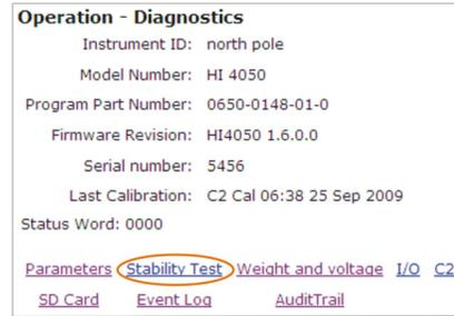
The results will not be specific to each load sensor, as in the IT test. They will display an average reading and PASS/FAIL for the system as a whole.
