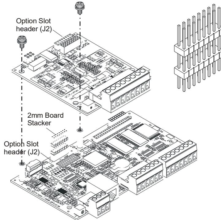
Step 3. Gently push the card onto the 20mm board stacker pins (making sure you align them through holes on the analog board with the two standoffs on the Main Controller board) until the pins are seated.
