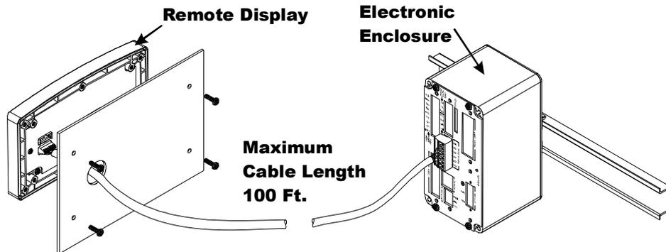
Step 4. Connect the cable wires to the display and the Electronic Enclosure.
