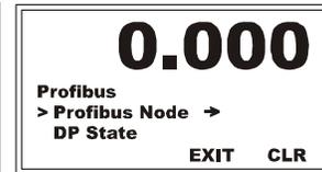
Step 3. Press CLR to clear the current entry and position the cursor, then use the up or down arrow to select the number for the right-most digit.
