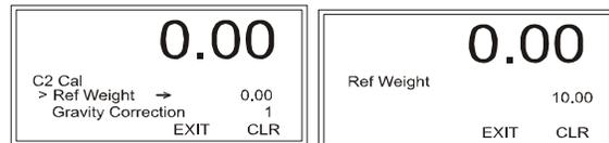
Step 4. Use the left or right arrow to position the cursor and the up or down arrow to select the value.
