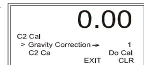
Step 6. Select Gravity Correction to open the edit page if you want to enter a gravity correction.
