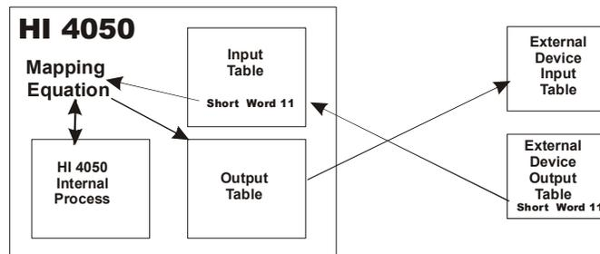
Often, more than two devices are involved, so separate input and output tables having different addresses may be set up for data exchanges with each device.
