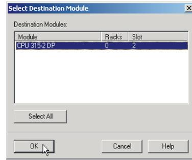
Step 10. Click OK to open the Select Station Address Dialog box; then click OK again. A status box will show the progress of configuration download to the PLC.
