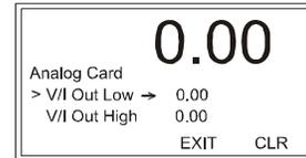
Step 4. Use the left or right arrow to position the cursor and the up or down arrow to select the value. When you finish, press Enter to save and return to the Analog Card menu.
