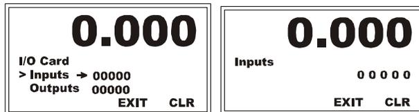
Step 3. The Inputs are displayed as a 5-bit value. (0 0 0 0 0). Note that the least significant (right-most) digit is input 1 and the most significant (left-most) digit is input 5. For example, with Input 1 and Input 3 active, the display reads.
