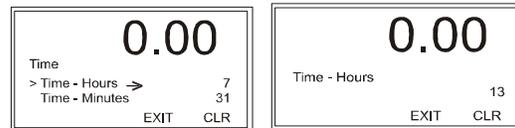
Step 11. Use the same procedure described for setting the month to set the hour using the 1-24 hour format.
