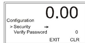
Step 2. Press Enter to open the Security Menu; then select High Password to display the High Password editing form.
