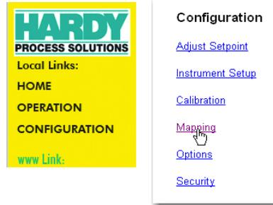
Step 2. Select Mapping to view the Configuration Mapping Setup form. The pull-down menus list both Destination and Source setup options.
