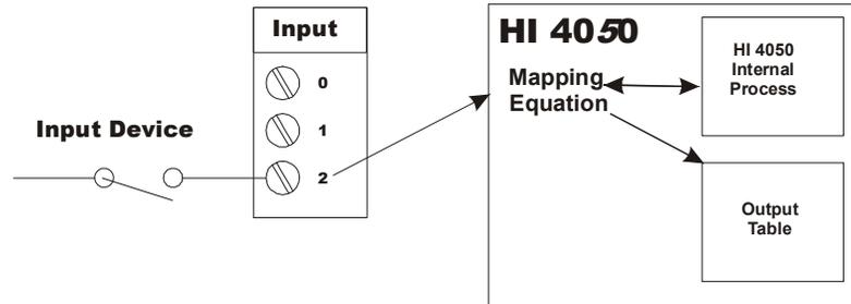
The source of such inputs would be an interface with a limit or selector switch, push button, or some other sensor feeding voltage signals into the HI 4050.
