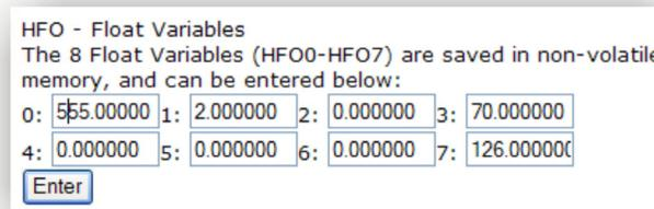
Step 11. On the Hardy Modbus-Link page Display pull-down menu, select Float Inverse. The value we entered from the Mapping page appears to the right of the "00000 =" which is 555.0000
