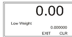
Step 6. Use the left or right arrow to position the cursor and the up or down arrow to select the value. When you finish, press Enter.
