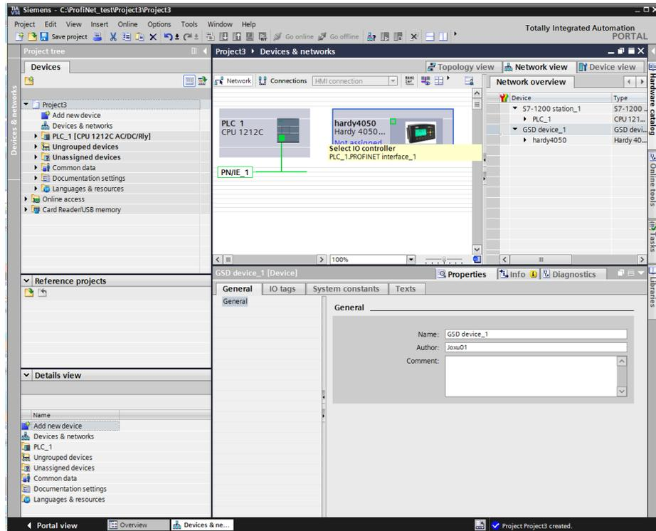
Step 8. As you added HI4050 to your PROFINET network, TIA Portal has been automatically assigning them DCP station name and IP addresses, this could make your network run with those default values. If you want to change the DCP station name and IP address from default for the HI4050 device, you also can assign your own DCP station name and IP addresses in your network using the steps below. NOTE: each device must have a unique DCP station name and IP address
