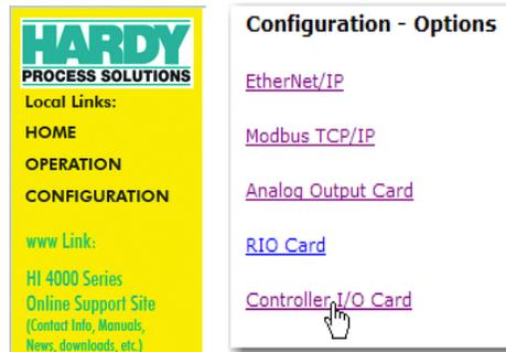
Select Controller I/O Card on the Options menu to open the read-only I/O Card page. This page shows the Inputs and Outputs that are currently activated. You may need to refresh your web screen to view any changes to the inputs.
