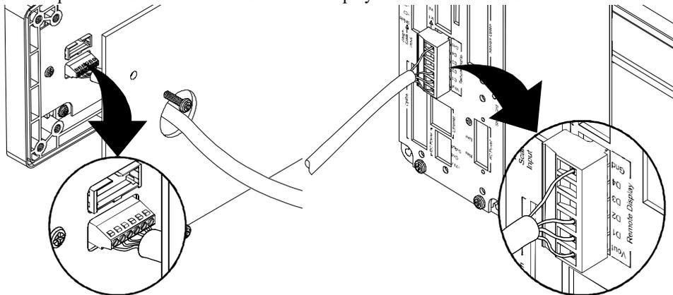
Step 5. Strip enough insulation off the cable wires so that you can connect the wires to The Electronic Enclosure and Remote Display connector.
