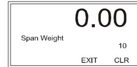
Step 8. Use the Down Arrow button to select Cal High, then press Enter to do the Cal High. A “Cal Completed OK” message appears briefly if the calibration is successful. An Error number appears if the calibration fails. See the Error list in Chapter 8, Troubleshooting for help with error correction.
