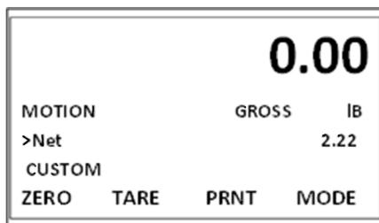
This display with the “>” is an indication that the scale reading is at 0.00 +/- .5 grad.
