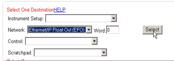
**NOTE** An address such as EFO2 means the following. EFO = EtherNet Float Out. 2 = Word 2.
