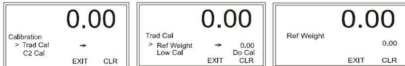
Step 2. Set the reference weight equal to the weight on the scale. Normally, you would remove all weight “live load” from the Scale to obtain a Ref Weight of 0.0. Wait 12 seconds or more for the reading to stabilize.
