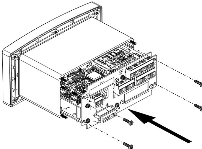
Step 3. Gently slide the circuit boards into the electrical enclosure until the rear panel is against the enclosure.
