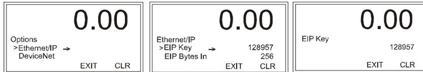
Step 2. Use the left or right arrow to position the cursor and the up or down arrow to select the values. Enter key number you received from the HI Service Center and press Enter to save it. Note that the number displayed above is only for illustration purposes and is based on the serial number.
