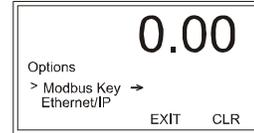
Step 2. Select Modbus Key to open the Modbus Key edit screen.
