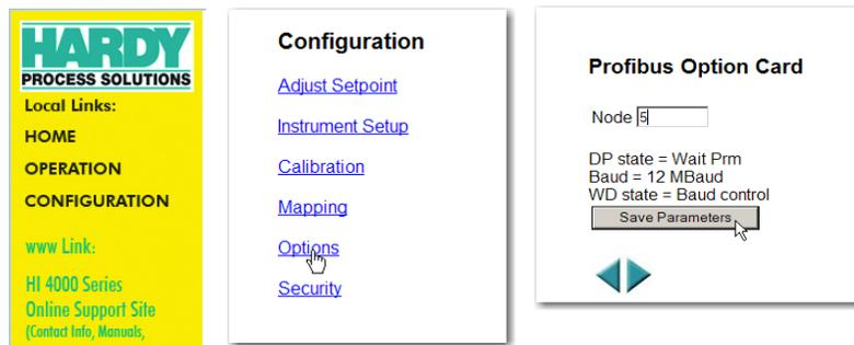
Double click in the Node text field to highlight the current entry. Type in the HI 4050 Node address. **Range:** 1-125 (default 5) Our example uses the default address #5.
