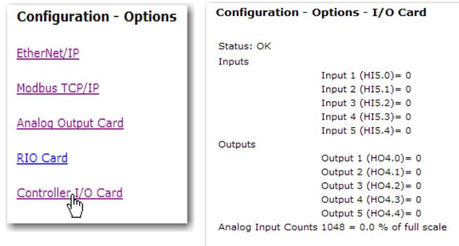
To test the inputs, continuously activate the input and refresh the web page while the input is activated. Confirm and move on to the next input. Be careful not to cause any false actions on the system while testing. When an input is activated you will also see the output percentage of full scale displayed at the bottom of the display.
