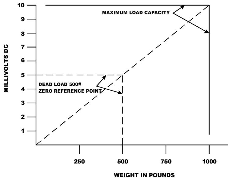
Based on this example, the operating range for this scale is 5-10 mVDC with a 500 pound weight. Understand that after zeroing the instrument the 0 reading on the instrument refers to the zero reference point and not absolute 0 mVDC or absolute 0 weight.
