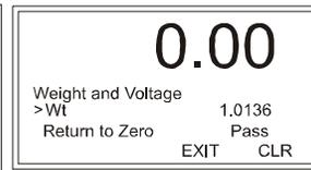
Step 1. To select a Sensor, use the up or down arrows to move through the list, and press Enter to display the sensor IT Test results for the selected sensor. Our example looks at Sensor number 1.
