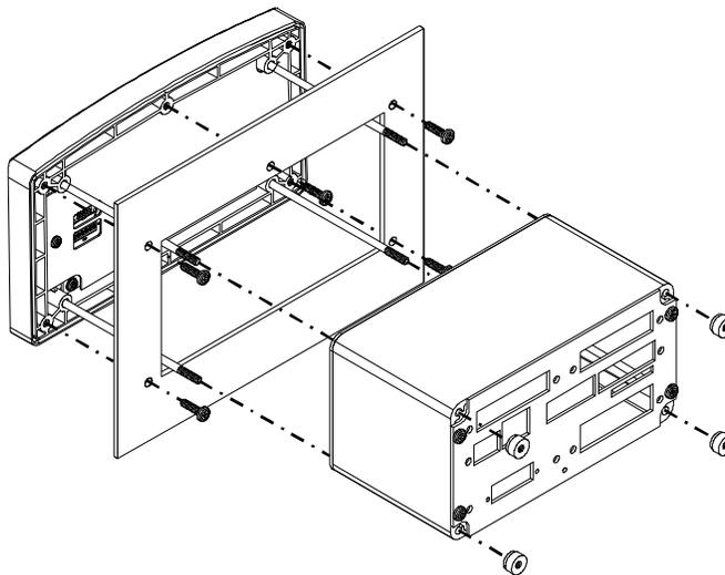
**Installing the Wall Mount HI 4050+ Weight Controller**
