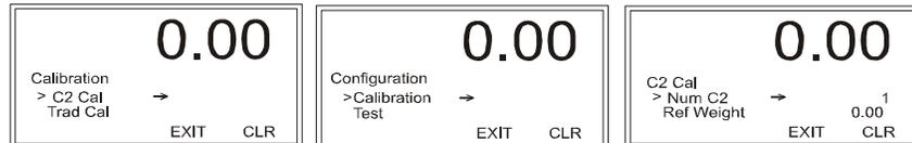
Step 2. The read-only Num C2 lists the number of C2 load cells on the system detected by the HI 4050. Verify that the displayed number matches the actual number installed. If not, check to ensure that each load cell/point cable connection is securely fastened and that each load cell/point cable is not broken.
