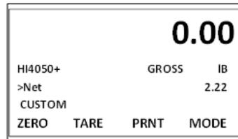
Below, the display of the unit indicates that the Scale connected to the HI 4050 is in motion.
