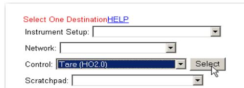
Step 2. When you click Select, the Control text box displays the destination address.
