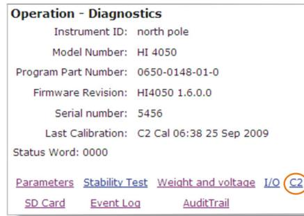
Step 2. From the Read Data from: pull-down list, select the C2 load sensor you want to view.
