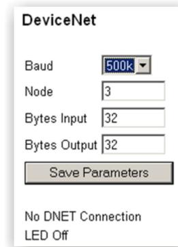
The screenshot shows the 'DeviceNet' configuration interface after saving. The fields are: 'Baud' with a dropdown menu showing '500k', 'Node' with a text field containing '3', 'Bytes Input' with a text field containing '32', and 'Bytes Output' with a text field containing '32'. A 'Save Parameters' button is located at the bottom of the form. Below the button, the status is displayed as 'No DNET Connection LED Off'.
