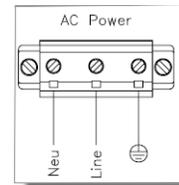
The HI 4050 is configured with a universal power supply rated from 120 to 240 VAC.
