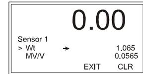
Step 3. Press the Exit button to return to the Sensor Menu. If you want to test other load sensors select the sensor and repeat steps 1 through 5 above.
