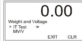
Then select IT Test to run the test. To read the rest of the results, press the down arrow. The weight and voltage/reading raw counts and average are shown below.
