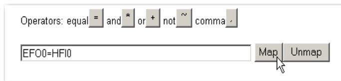
Step 7. Click Map to complete the Gross Weight to EtherNet/IP Float Out equation. The Gross Weight that is stored in the input table is now assigned to the EtherNet/IP Float Out output table and to the EtherNet/IP Network. The Map list, shown below, shows the new mapping.
