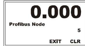
Step 4. Press the left arrow to move the cursor to the next digit, and use the up or down arrow to select the number for the left digit. Our example sets the Node Address at #7.
