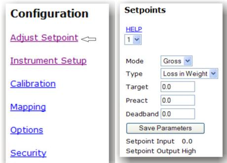
**Step 1.** If your system uses more than one setpoint (up to four may be used), you will need to know which one you should change. To select the Setpoint to configure, use the pull-down list below Help. In our example we selected Setpoint 1, which appears in the text field.
