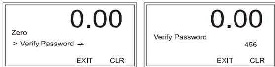
Step 8. Press Enter to display the Verify Password edit screen. Use the up or down arrows to enter the assigned password (for either High or Medium Passwords) and press Enter. The Zero process can then proceed and you are returned to the Security Menu. Since we assigned a Medium Password of 456, we would enter 456.
