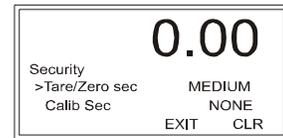
To Tare or Zero the instrument you need a password. When you Tare or Zero the instrument, Verify Password appears.
