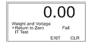
FAIL indicates that you are outside the sum of the preset Motion and Zero Tolerance settings. If this results from too much build up on the scale, you need to clean the scale or you have scale problems. Run this test whenever you cannot zero the scale. If the Return to Zero test fails, see the E Flow Char - Non Return to Zero for troubleshooting help.
