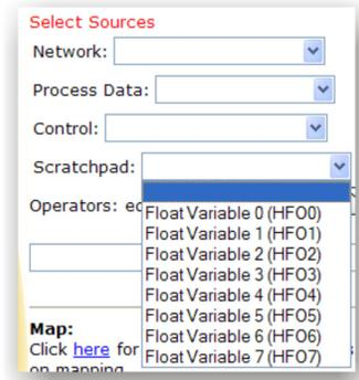
Step 9. Click Map to complete the mapping (Float Variable 0, word 0 to Modbus Float Out, Word 0).
