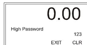
Step 3. Use the left or right arrow to position the cursor and the up or down arrow to select the value. When you finish, press Enter to save the password and return to the Security Menu. Our example shows 123 (*for illustration only*).
