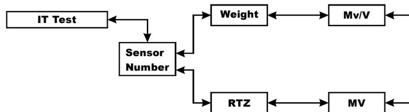
If your system has an Integrated Technician Summing Junction box, the IT test can help identify individual load cell problems up to a maximum of four load cell selections.
