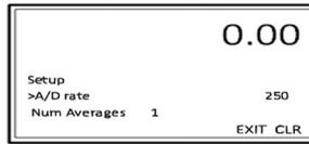
**On the 4050+ Display:** From the Setup Menu, arrow down to select A/D rate. Toggle between 110 or 250 to make your selection and hit Arrow down to Enter to select the desired rate.
