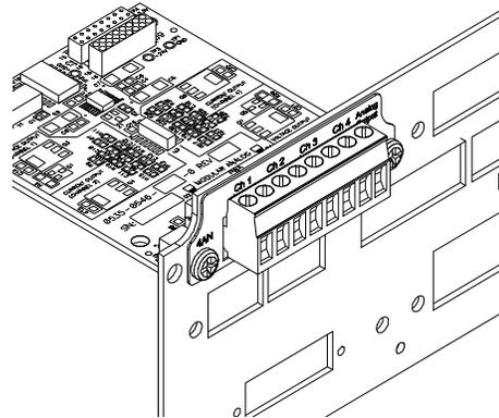
**WARNING - The Voltage and Current outputs are not interchangeable. To interchange voltage and current will cause personal injury and/or property damage.**
