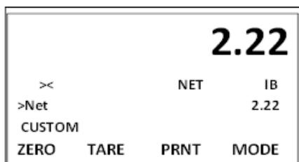
Pressing the MODE button will change the large number display between GROSS, NET, And ROC (if enabled) as show here with NET Selected.
