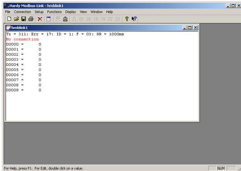
Step 2. Click Connect in the Connection pull-down menu, to display the TCP/IP Connection form.
