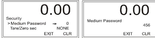
Step 5. Use the left or right arrows to select a digit and the Up or Down arrows to scroll to the value, and press Enter to save and return to the Security Menu. To delete an entry, use the left arrow. Our example (*for illustration only*) shows 456.
